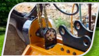
Orbit motor hydraulic system and check valve to protect the motor.
