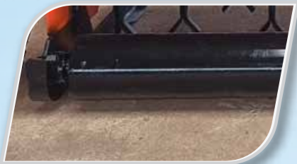
Special rear roller to protect blades during operation.
