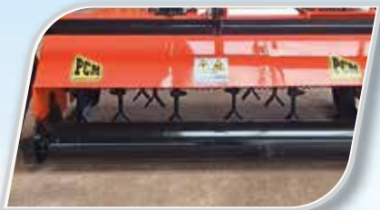
Skid shoes for adjustable cutting height (3 levels).
