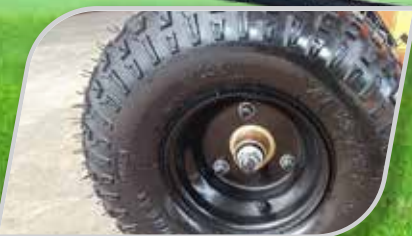
Special rear wheels designed to prevent punctures and improve access to tree bases.
